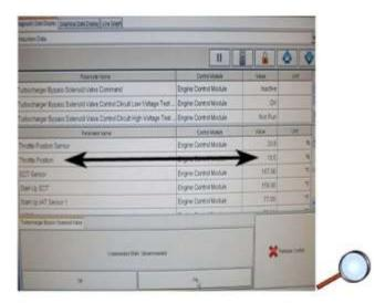
If normal SI diagnosis does not resolve DTC P1101, check the throttle position angle. A good throttle position at idle should be between 8-12%. Make sure the engine is warm and the A/C or defrost mode is OFF.
